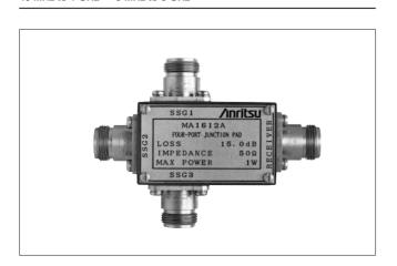
The MP659A and MA1612A are used as an impedance matching box applying the mixed output of three RF signal generators to a receiver input terminal for measurement of three-signal characteristics (such as receiver SINAD performance).
